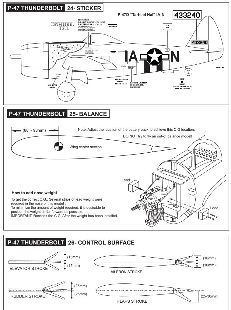
Adjust the travel of the control surfaces to achieve the values stated in the diagrams. These value will be suitable for average flight requirements. Adjust the values to suit your particular needs.
