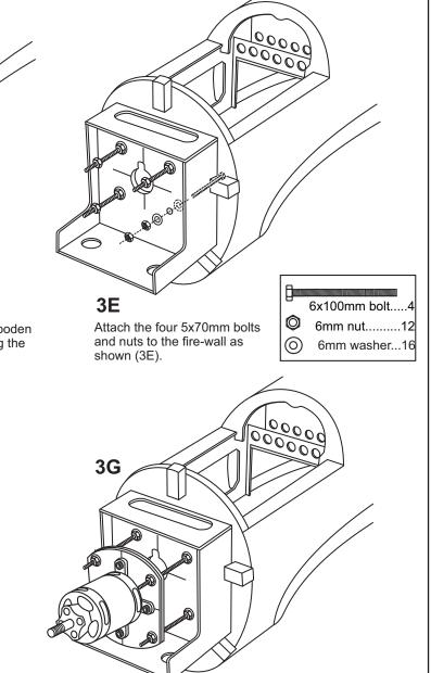
Remove the wooden motor mounting plate and drill a 6mm hole through the fire-wall at each of the four marks marked (3D).
