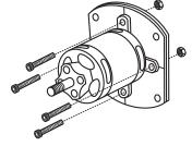
Secure the Motor to the wooden motor mounting plate using the four 3mm bolts.
